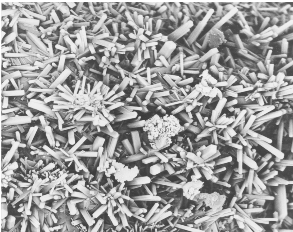
Figure 1 Micrograph showing elongated fluorapatite crystals.
